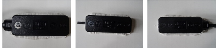
Fig. 7: View of junction box of module type SE4-72H-450M
